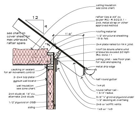
E1 Typical Exposed Eave rafters on joist
